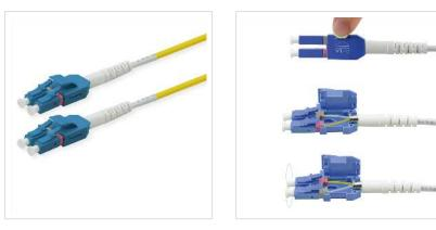
ROLINE Fiber Optic Uniboot LSOH Patch Cord LC/LC in OS2 quality. A uniboot connector is ideal for a high-density environment. Compared to conventional duplex patch cords, the design is more compact and only one cable is used for two lines, which enables usage in a high-density environment. Changing the fiber polarity is easily possible without special tools.
