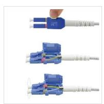
ROLINE Fiber Optic Uniboot LSOH Patch Cord LC/LC in OS2 quality. A uniboot connector is ideal for a high-density environment. Compared to conventional duplex patch cords, the design is more compact and only one cable is used for two lines, which enables usage in a high-density environment. Changing the fiber polarity is easily possible without special tools.
