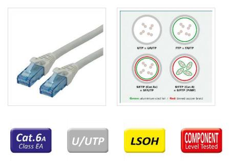
Patch cable for networking connections between devices. Prepared unshielded Twisted Pair cable with RJ-45 connectors on both ends. Durable due to moulded kink protection. Flexible cable, suitable for narrow bending. High quality plugs with gold plated contacts. Contact settings 1:1, in accordance with the EIA/TIA 568 standard. Construction: 4-pair stranded copper wire.
