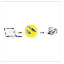
• For connecting a PC/notebook equipped with USB Type C port to a peripheral device with a USB 2.0 Type B port (e.g. printer/scanner or an external hard disk HDD)
