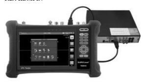
DVR or other device's HDMI out port connect to tester's HDMI in port, the meter will display input image.
