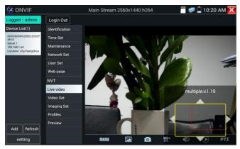
When the image is enlarged, if not operate on touch screen, it can operate by the keyboard, press the key (TELE+) to zoom in, press the key (WDE-) to zoom out, press upward and downward key to move image. If it is network video input to the tester, as the tester supports resolution up to 1080p, the input image will be very clear after it is enlarged. This is greatly helpful for the installers to ensure the IP camera's video coverage and decide the IP camera's install site.
