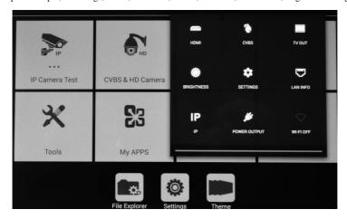
**HDMI:** Click HDMI to enter HDMI IN mode, it can converts test from analog to digital with dual test window IP & HDMI IN or Analog & HDMI IN.
