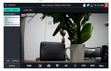
**IP camera video settings:** Click "Video Set" to enter the IP camera's encoder and resolution settings. Make the desired changes and click "OK "to save.
