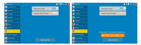
Start the FTP server and then input the tester's FTP address in the PC's address bar. This will enable the PC to reads, copy and edit the files from the SD card without the use of SD card reader.
